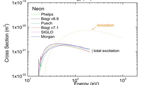
Ionization and sum of inelastic cross sections
